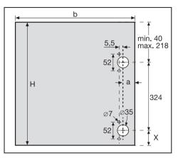
if width (**b**) increases, measurement **a** must also be increased
